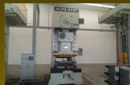
► 冲床切边 punch machine for trimming
